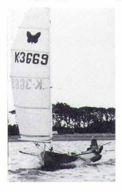
A very successful year for this design which is a refinement of the earlier Sprite. Built with greater freeboard and rig moved further aft, it has a shallow V underwater shape with a moderate amount of rocker and a single hard chine above the waterline. Wings are tubes and trampolines and there is a foot well cockpit with bailer. A good boat in all weathers, it is exceptional upwind in the stronger breezes.
