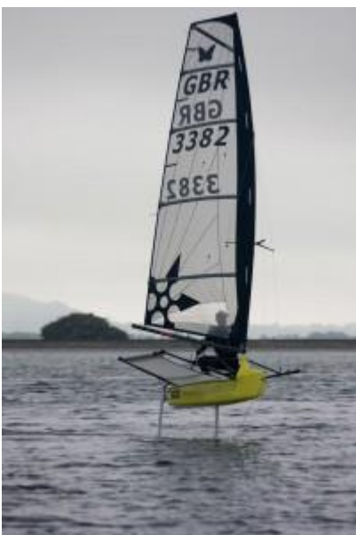
Photo 3. Mike Cooke in light winds in the 'About to Gybe' Position, kneeling on the front leg and with the back foot placed on the hull.
