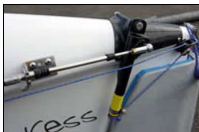
Bow of a Prowler Moth showing the ride height adjustment mechanism.
